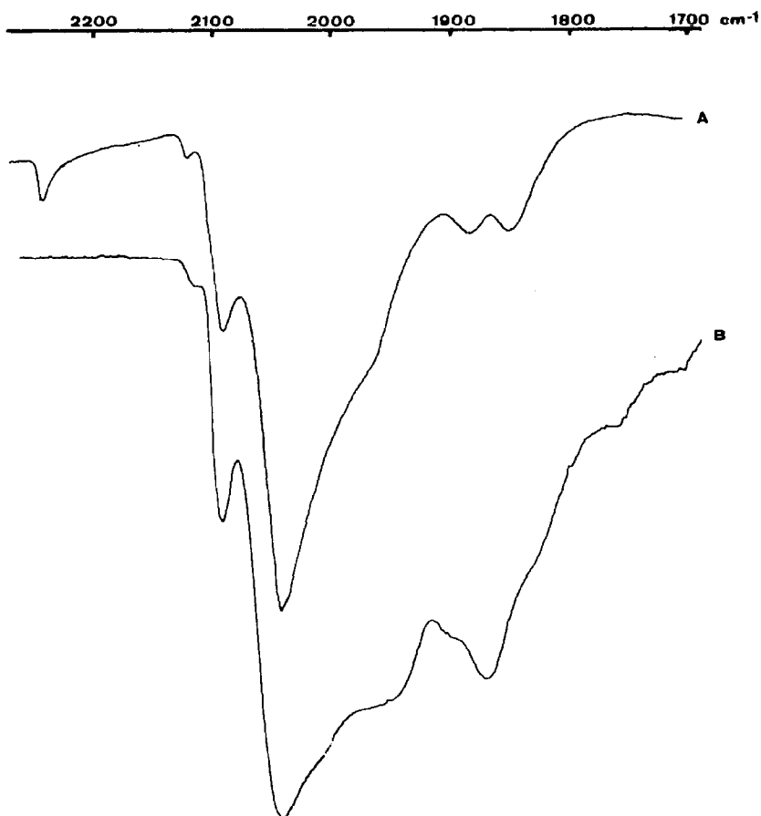
Fig. 4. Spectra of [\text{HFeCo}_3(\text{CO})_{12}] adsorbed (by deposition from the gas phase) on \text{Al}_2\text{O}_3 (A) and on MgO (B).
