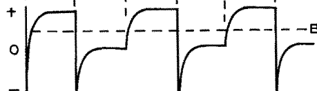
Fig. 1. A: output signal (at point x ) averages to zero for long time constant; B: output signal (at point y ) averages to \sim \frac{1}{2} maximum value for long time constant; "on" and "off" refer to the UV light; Output signal: ——— short time constant. - - - - - long time constant.
