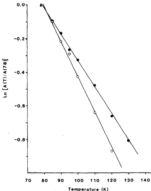
Fig. 1. Variable temperature Mössbauer spectroscopic data for  $(\text{Me}_3\text{Sn})_2\text{pdtc}$  (○) and  $\text{Me}_2\text{Snpdtc}$  (●). Data for the former are  $a 2.12 \times 10^{-2} \text{ K}^{-1}$ , ( $78 \leq T \leq 120$ ), correlation coefficient  $r -0.997$  (7 pts) and the later  $a 1.58 \times 10^{-2} \text{ K}^{-1}$  ( $78 \leq T \leq 130$ ),  $r -0.999$  (8 pts). The point  $\blacktriangle$  (78, 0.0) is common to both plots.
