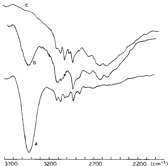
Fig. 2. IR spectra of complex IIa in \text{CH}_2\text{Cl}_2 solution (OH group absorption): a, recorded immediately after formation; b, after storage for 12 h; or c, for 24 h.
