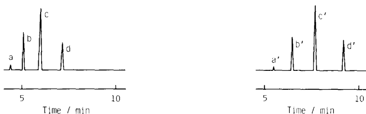
Fig. 1. Gas chromatogram of the solution (HMDS/MTEOS ratio of 3.0) which has been treated with Amberlyst 15 at 40 °C for 85 h.
