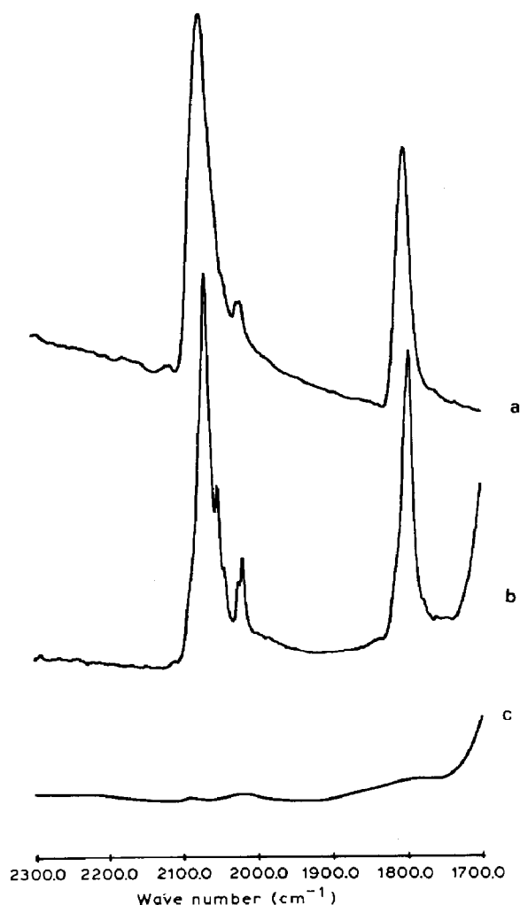
Fig. 1. Infrared spectra in the \nu(\text{CO}) region ( \text{cm}^{-1} ): (a) \text{Rh}_6(\text{CO})_{16} in KBr; (b) \text{Rh}_6(\text{CO})_{16} supported onto a \text{MgO}_{\text{air}} ; (c) as (b), after 1 h in vacuo at 80^\circ\text{C} and further 24 h under CO at 25^\circ\text{C} .
