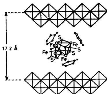
Fig. 6. Representation of the cluster bronze  $[\text{MoO}_3\{\text{Fe}_4(\eta\text{-C}_5\text{H}_4\text{Me})_4(\mu_3\text{-S})_4\}_{0.15}]$ .
