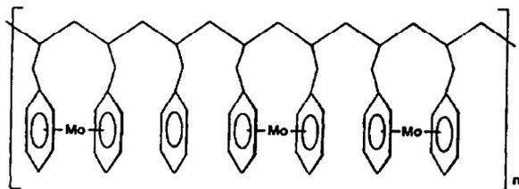
Fig. 11. Ladder polymer of bis( $\eta$ -allylbenzene)molybdenum.
