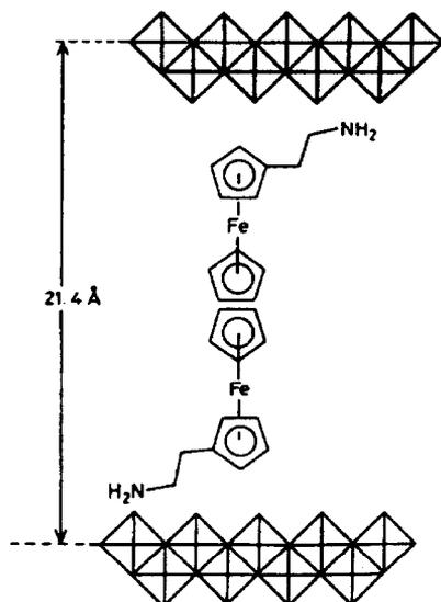
Fig. 7. Representation of the intercalate  $[\text{MoO}_3(\text{Fe}(\eta\text{-C}_5\text{H}_4\text{CH}_2\text{CH}_2\text{NH}_2)(\eta\text{-C}_5\text{H}_5))_{0.05}]$ .
