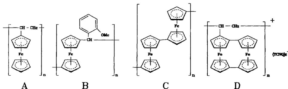
Fig. 10. Examples of some ferrocene based organometallic polymers.
