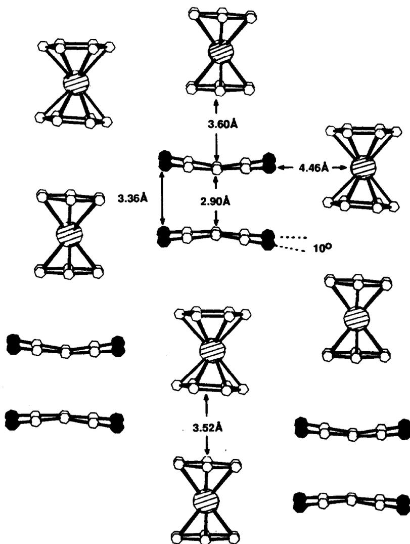
Fig. 2. Molecular structure of  $[\text{Cr}(\eta\text{-C}_6\text{H}_6)_2]^+[\text{TCNE}]^-$ .
