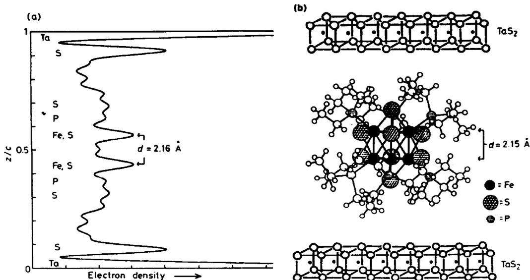
Fig. 5. (a) Projection of the electron density of  $[\text{TaS}_2\{\text{Fe}_6\text{S}_8(\text{PET}_3)_3\}_{0.05}]$  along the  $c$ -axis. (b) Schematic illustration showing the orientation of the iron cluster between the  $\text{TaS}_2$  layers, as deduced from the interlayer electron density.
