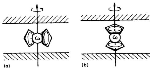
Fig. 8. Proposed models for TaS<sub>2</sub>-metalloocene intercalation compounds, with the principal axis (a) parallel to and (b) perpendicular to the interlamellar plane.
