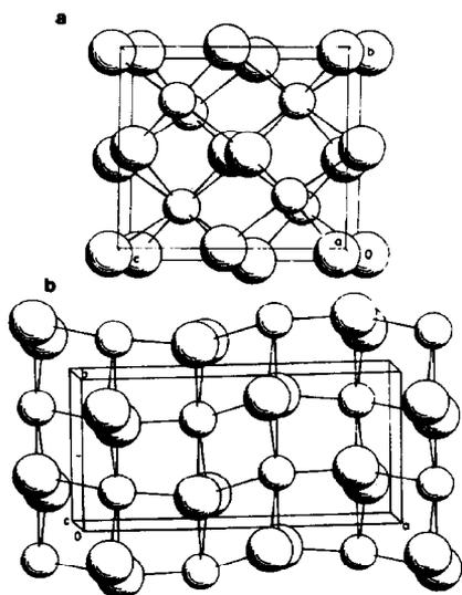
Fig. 4. Molecular packing of the "soft salt"  $[\text{Mo}_4(\eta\text{-C}_5\text{H}_4\text{Pr}^i)_4(\mu_3\text{-S})_4]_2^+ [\text{Os}_6(\text{CO})_{18}]_2^-$  in its two alternative monoclinic forms (a) and (b). The larger spheres represent cations and the smaller anions.
