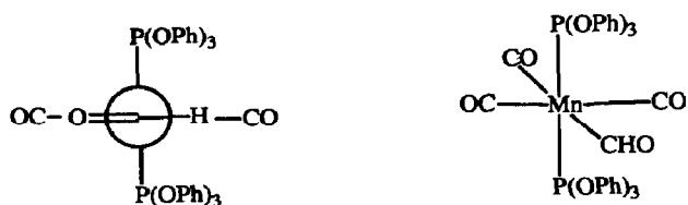
Fig. 10. Newman projection derived from the X-ray crystal structure of [\text{Mn}(\text{CO})_2(\text{P}(\text{OPh})_3)_3\text{CHO}] ( \theta = 179^\circ , \nu(\text{C}=\text{O}) = 1585 \text{ cm}^{-1} ).
