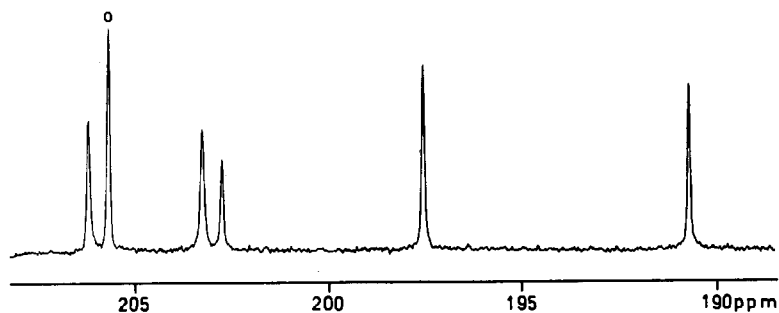
Fig. 2. ^{13}\text{C}\{^1\text{H}\} NMR spectrum (acetone- d_6 , 75.5 MHz, -85^\circ\text{C} ) of a ^{13}\text{C} -enriched sample of [\text{Ru}_6(\mu_4\text{-Hg})(\mu_3\text{-ampy})_2(\text{CO})_{18}] ( 2 ). The peak marked with a circle comes from the solvent.
