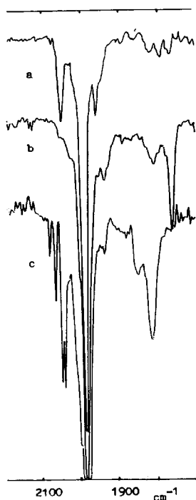
Fig. 1. IR spectra in cyclohexane of \text{HRh}(\text{CO})(\text{PPh}_3)_3 + \text{Rh}(\text{acac})(\text{CO})_2 (1:1) (a, b) and \text{HRh}(\text{CO})(\text{PPh}_3)_3 + \text{Rh}(\text{acac})(\text{CO})_2 (1:2) (c) mixtures. (a), (c) immediately after mixing; (b) after 5 min.
