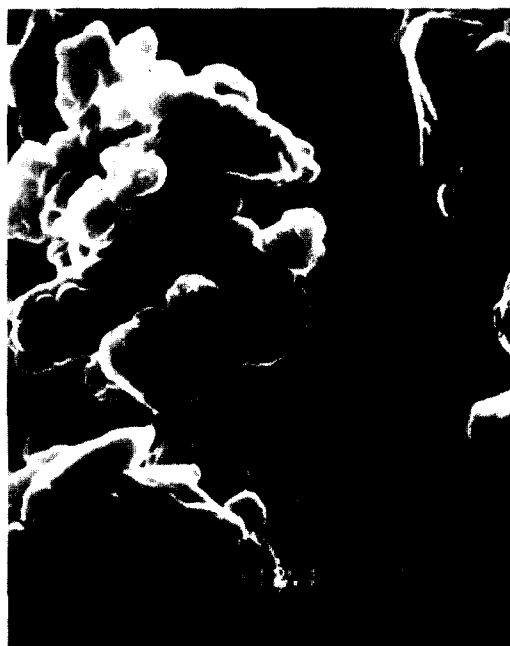
Fig. 2. SEM for AlN derived from [\text{HAlNH}]_n .
