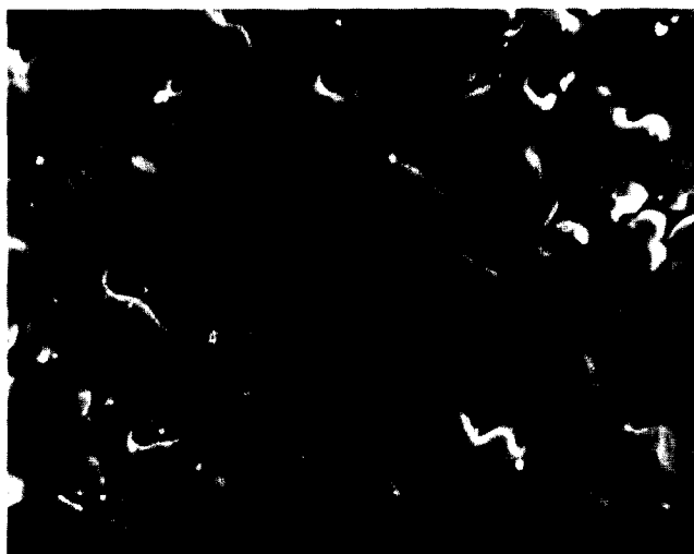
Fig. 4. Scanning electron micrograph at 15 kV showing the morphology of the silver film obtained by MOCVD from trans - [CF_3CF=C(CF_3)Ag]_4 ( 1 ) at 275°C.
