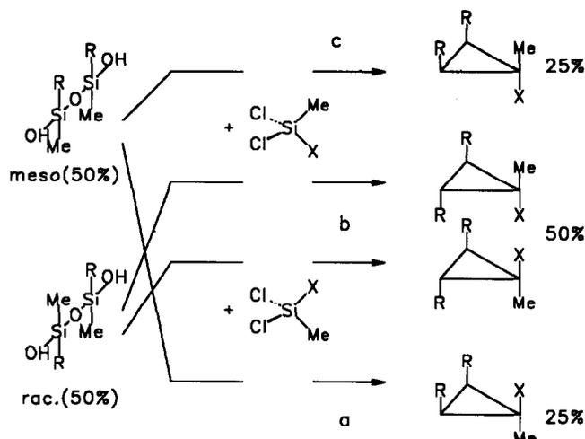
Scheme 1. Formation of configurational isomers in the synthesis of cyclotrisiloxanes [(RMeSiO)<sub>2</sub>(XMeSiO)], with statistical isomeric distribution.
