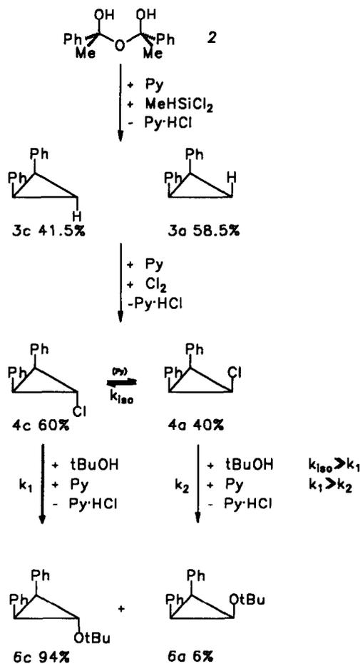
Scheme 2. Route to 2-*t*-butoxy-2,4,6-trimethyl-4,6-diphenyl-(2 $\alpha$ ,4 $\beta$ ,6 $\beta$ )-cyclotrisiloxane.
