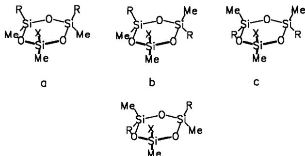
Fig. 1. Structure of the three configurational isomers a–c of cyclotrisiloxanes. 3: R=Ph, X=H; 4: R=Ph, X=Cl; 6: R=Ph, X=O<sup>t</sup>Bu.
