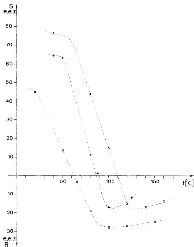
Fig. 1. Asymmetric hydroformylation of styrene in the presence of  $\text{PtCl}(\text{SnCl}_3)(\text{BDPP})$  in toluene (+);  $\text{PtCl}_2(\text{BDPP}) + \text{SnF}_2$  in toluene (x) and  $\text{PtCl}_2(\text{BDPP}) + \text{SnCl}_2$  in dichloromethane (o).
