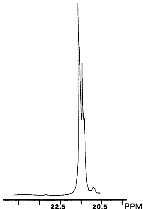
Fig. 2. Methyl resonances in the ^{13}\text{C} NMR spectrum of poly(( Z )-pentadiene) obtained with [\text{CpTiCl}_3]\text{-MAO} . The peak at 21.632 ppm is attributable to mm triads, that at 21.490 ppm to mr triads [8]. ( \text{C}_6\text{D}_6 ; room temperature; TMS as internal standard.)
