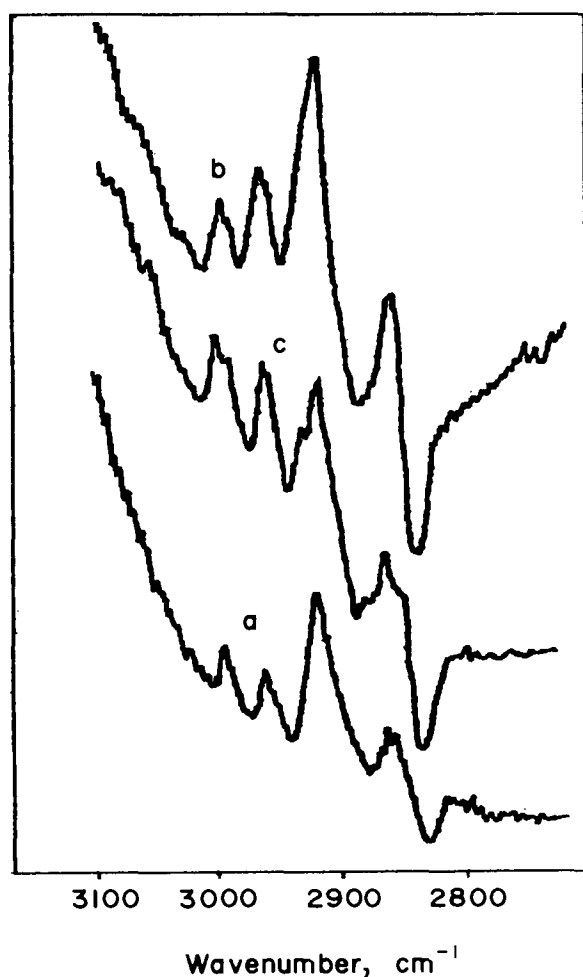
Fig. 3. The IR spectra of aerosil surface products obtained in course of the reactions between (a) SC and ethylene oxide; (b) surface silanones and ethylene oxide; (c) surface sila-dioxiranes and ethylene. Gaseous reagent pressures were no more than 5 \cdot 10^{-2} Torr.
