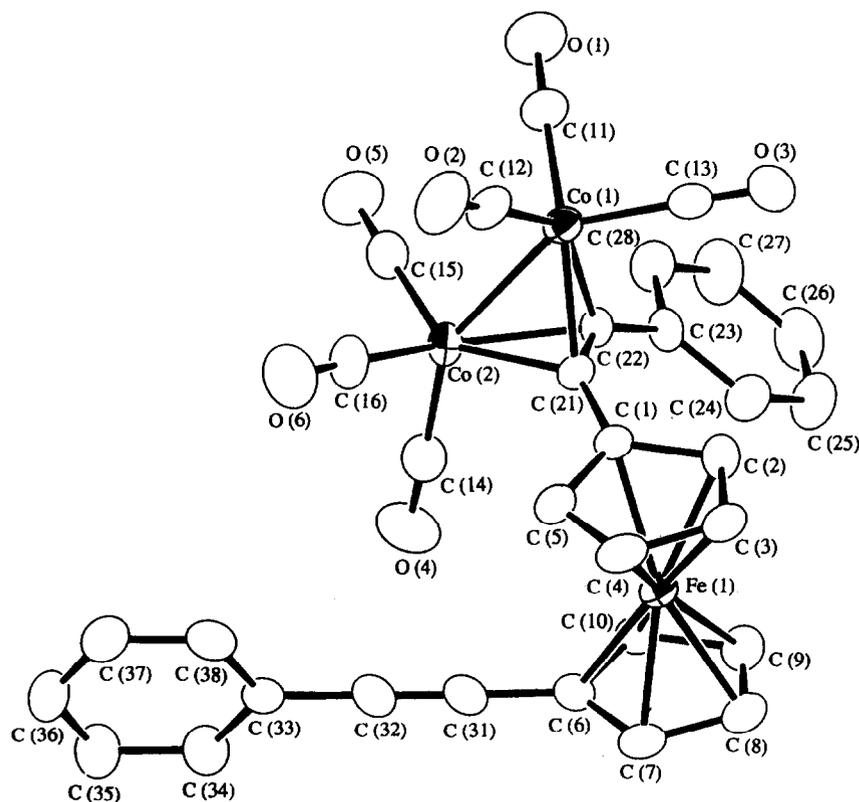
Fig. 2. ORTEP drawing of  $\{(\eta^5\text{-C}_5\text{H}_4\text{C}\equiv\text{CPh})_2\text{Fe}\}\text{Co}_2(\text{CO})_6$  (**4**). The non-hydrogen atoms are represented by 30% probability thermal ellipsoids, and the hydrogen atoms are omitted for clarity.
