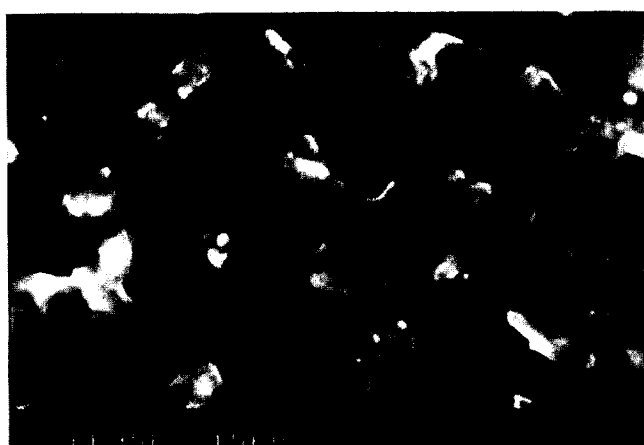
Fig. 8. Scanning electron micrographs of \beta -CoGa (film no. 3, Table 4) at two magnifications, showing pits due to thermal decomposition of the GaAs surface.
