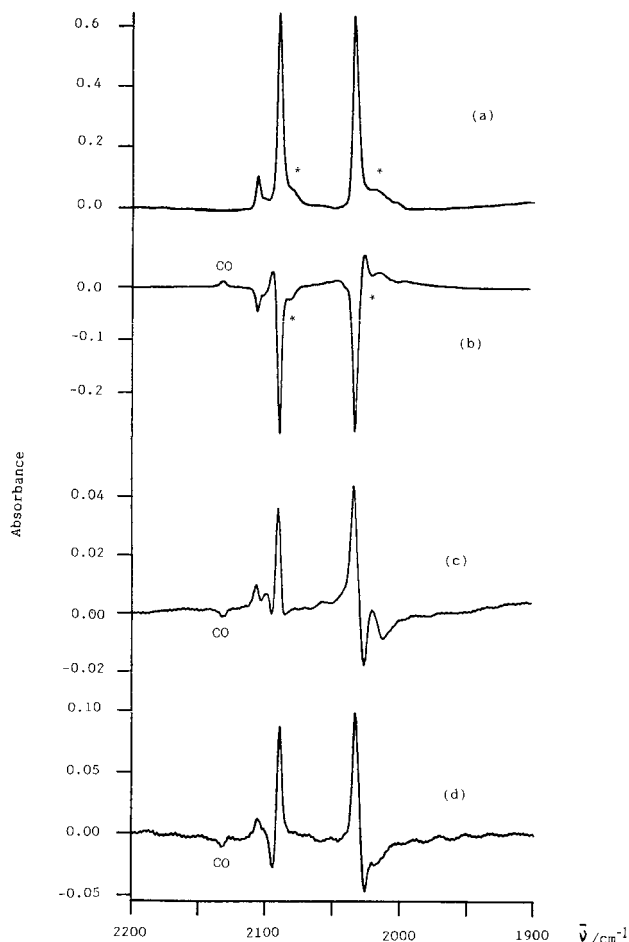
Fig. 5. I.r. spectra from an experiment with \{\text{Rh}(\text{Cl})(\text{CO})_2\}_2 dispersed in a Nujol mull: (a) at 77 K, (b) after 30 min mid-UV irradiation (filter D) minus starting material (subtraction spectrum (b), A(a) where A is a scaling factor); (c) after 45 min back photolysis (filter C); (d) after annealing the mull to -100^\circ\text{C} minus back photolysis (subtraction spectrum (d), C(c) where C is a scaling factor). Bands marked * correspond to \text{Rh}_2(\text{Cl})_2(^{12}\text{CO})_3(^{13}\text{CO}) present in natural abundance.
