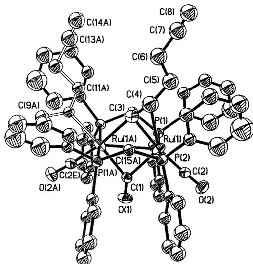
Fig. 3. A view of the structure of complex **8c**. There is a crystallographic two-fold axis passing through the  $\mu\text{-CO}$  group and only one of the resulting disorder forms is shown.
