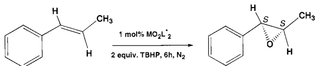
Scheme 3. Epoxidation of trans -methylstyrene (M = Mo, W).
