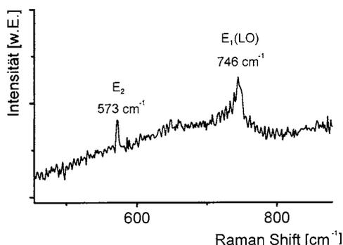
Fig. 6. Raman data of the GaN layer of Fig. 5. The characteristic absorption of bulk GaN, the  $E_2$  and  $E_1$  mode of the lattice vibration are clearly seen.
