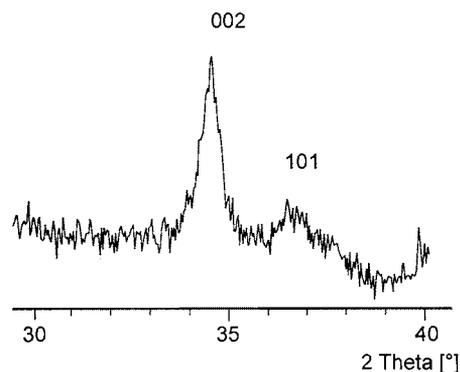
Fig. 5. Thin film X-ray diffraction pattern of a preferentially oriented crystalline GaN layer grown on *c*-plane sapphire using (N<sub>3</sub>)<sub>2</sub>Ga[N(CH<sub>2</sub>CH<sub>2</sub>NEt<sub>2</sub>)<sub>2</sub>] in vacuo at 750°C.
