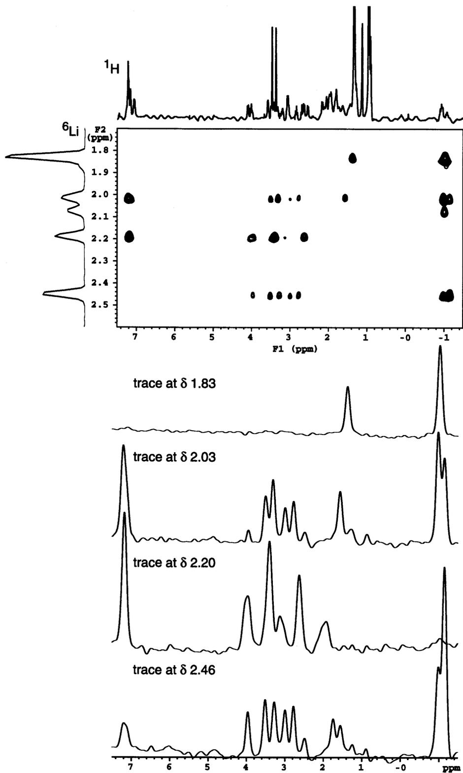
Fig. 4.  ${}^6\text{Li}$ ,  ${}^1\text{H}$ -HOESY NMR in  $\text{DEE-}d_{10}$  at  $-60^\circ\text{C}$  for Li-2 with three equivalents of *n*-BuLi in excess showing the  ${}^6\text{Li}$ -NMR traces at  $\delta$  1.83, 2.03, 2.20, and 2.46 ppm.
