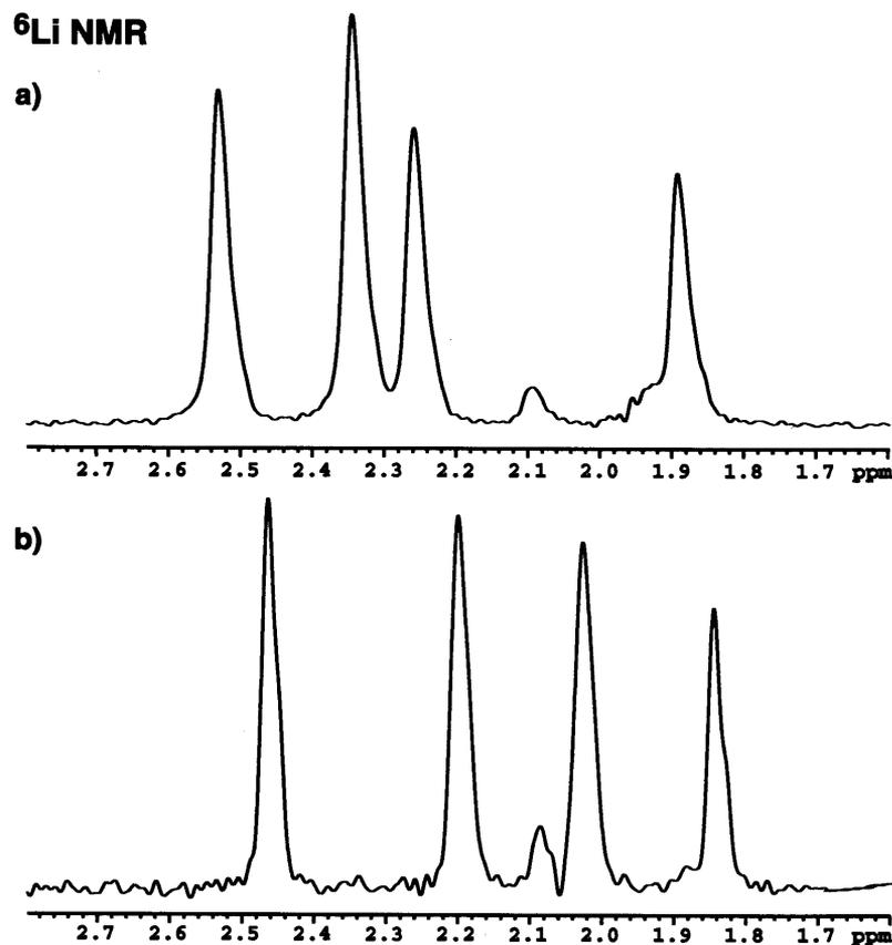
Fig. 2.  ${}^6\text{Li}$ -NMR in  $\text{DEE-}d_{10}$  at  $-60^\circ\text{C}$  of (a) Li-1 with two equivalents of  $n\text{-BuLi}$  in excess, (b) Li-2 with three equivalents of  $n\text{-BuLi}$  in excess.
