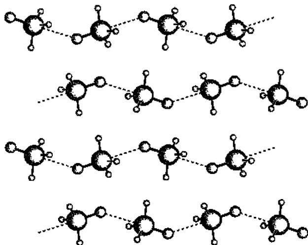
Fig. 2. The orientation of  $\text{FSiH}_3$  molecules within the crystal. Note the close intermolecular contacts between the large spheres (representing Si atoms) and the medium sized spheres representing the F atoms.
