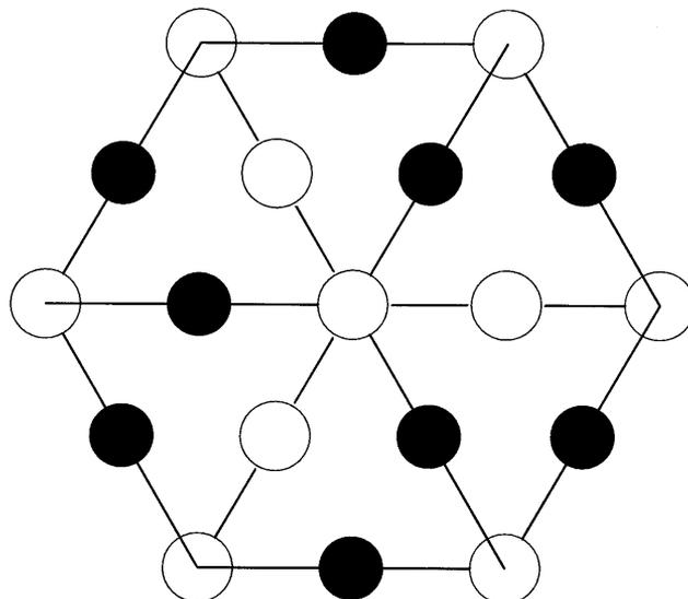
Fig. 11. The cubic NaCl-type lattice of KSiH<sub>3</sub> (black spheres are formal K<sup>+</sup> atoms, white spheres represent the [SiH<sub>3</sub>]<sup>−</sup> group: this figure was generated from data given in Ref. [28]).
