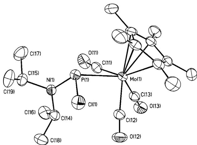
Fig. 2. Structural diagram of  $[\text{Cp}^*\text{Mo}(\text{CO})_3(\text{P}(\text{Cl})\text{N}^i\text{Pr}_2)]$ . Thermal ellipsoids are shown at the 50% probability level. Hydrogen atoms have been eliminated for clarity.
