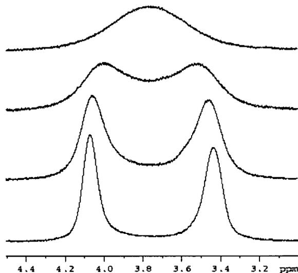
Fig. 1. Variable temperature  $^1\text{H-NMR}$  spectrum of  $[\text{Cp}^*\text{Mo}(\text{CO})_3(\text{P}(\text{Cl})\text{N}^i\text{Pr}_2)]$  (**1**), showing the coalescence of the isopropyl methylene hydrogen atoms. Temperatures shown are 35, 45, 55 and  $65^\circ\text{C}$ .
