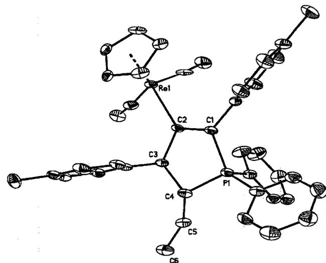
Fig. 4. X-ray crystal structure of  $\text{Cp}(\text{CO})_2\text{Re}[\text{C}=\text{C}(\text{Tol})\text{PPh}_2\text{CH}(\text{CH}=\text{CH}_2)\text{CH}(\text{Tol})]$  (**9c**).  $\text{Re}(1)\text{--C}(2)$  2.125(5) Å,  $\text{C}(1)\text{--C}(2)$  1.401(8) Å.
