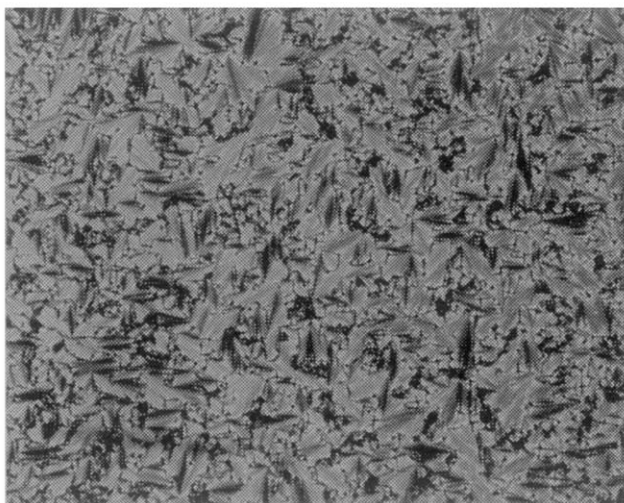
Fig. 2. Optical texture (200 ×) observed on cooling from the isotropic phase for imine ligand 2c : S 1 (S C ) phase at 70.2 °C (top) and copper(II) complex 3c : S 2 (S A ) phase at 106.4 °C (bottom).
