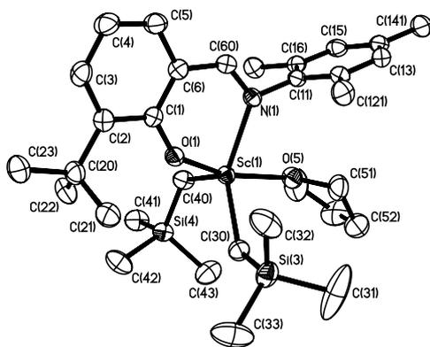
Fig. 1. Molecular structure of  $Sc(CH_2SiMe_3)_2(THF)(L^1)$  (**1**), showing the atomic numbering scheme. Ellipsoids are drawn at 50% probability.
