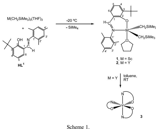
The NMR spectra in  $C_6D_6$  at room temperature indicate  $C_s$  symmetry of the complexes. While this work was in progress, Piers et al. reported the synthesis of sterically more hindered complexes  $M(CH_2SiMe_2Ph)(N-O)_2$  ( $M = Sc, Y$ ) bearing  $N-C_6H_3Pr^i$  substituents which undergo cyclometallation reactions [16].
