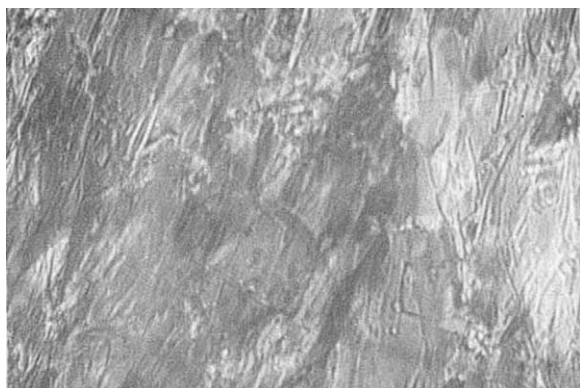
Fig. 3. Texture of the complex 3b under crossed polarizers, 124 °C, upon heating, \times 250 N phase.
