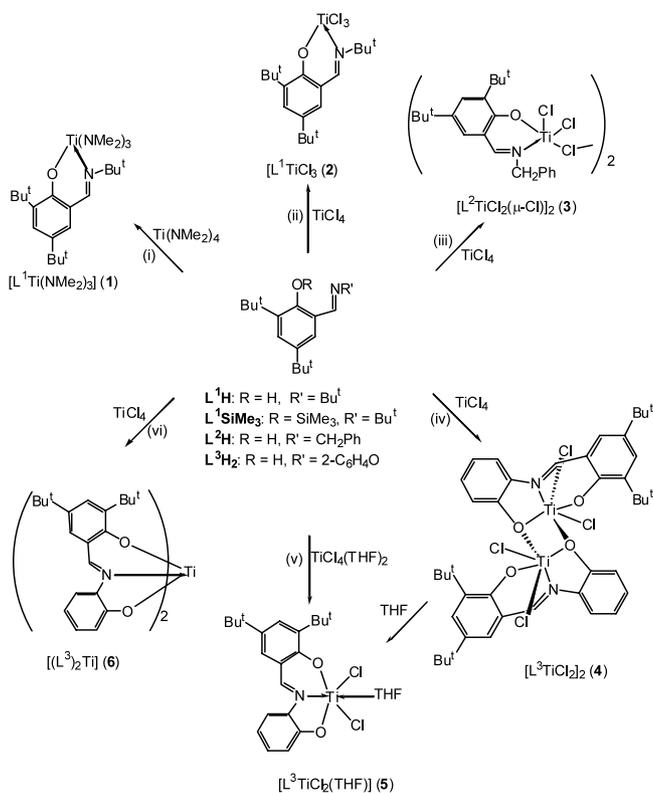
(i) **L<sup>1</sup>H** (1 equiv); (ii) **L<sup>1</sup>SiMe<sub>3</sub>** (1 equiv); (iii) **L<sup>2</sup>H** (1 equiv); (iv) **L<sup>3</sup>H<sub>2</sub>** (1 equiv); (v) **L<sup>3</sup>H<sub>2</sub>** (1 equiv); (vi) **L<sup>3</sup>H<sub>2</sub>** (2 equiv).
