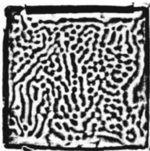
Figure 2. Mixed mosaic pattern of stripes and spots formed by Marangoni convection in a 2 mm solution layer. The dark color corresponds to the oxidized form and the white regions to the reduced form of Methylene Blue. Initial concentrations in the reaction chamber are [MB^+]_0 = 3.0 \times 10^{-4} M, [Na_2S]_0 = 2.1 \times 10^{-2} M, and [Na_2SO_3]_0 = 1.0 \times 10^{-3} M. T = 22 °C.
