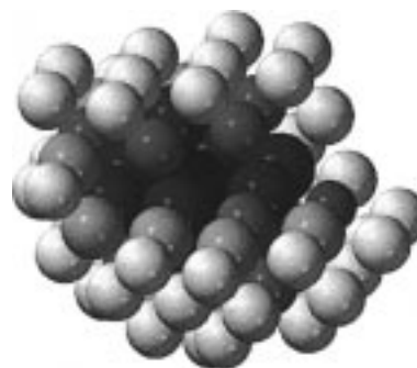
Figure 4. Final kinetic energy values of the ions gain in the Coulomb explosion process are indicated by different gray scales. The lighter the color, the more kinetic energy this ion gains during the Coulomb explosion. The dark colored ions located in the center of the cluster are those gaining the least kinetic energy.
