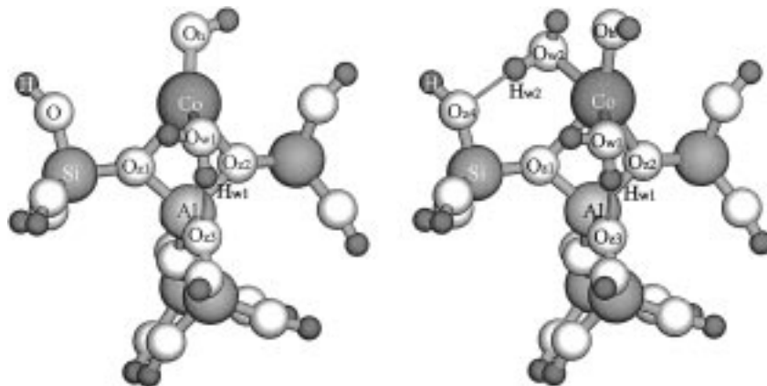
Figure 7. Structure of one and two waters bound to Co 2+ (OH) - Z - .
