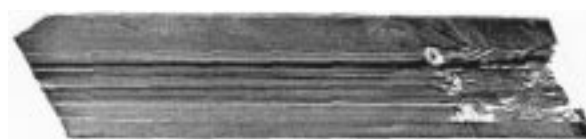
Figure 4. Thin section topograph of a solution-grown S3MeMBANP crystal with (010) as the input face. The seed is clearly seen on the right, and the growth dislocations arising from the seed are manifested by horizontal lines as the crystal grows.
