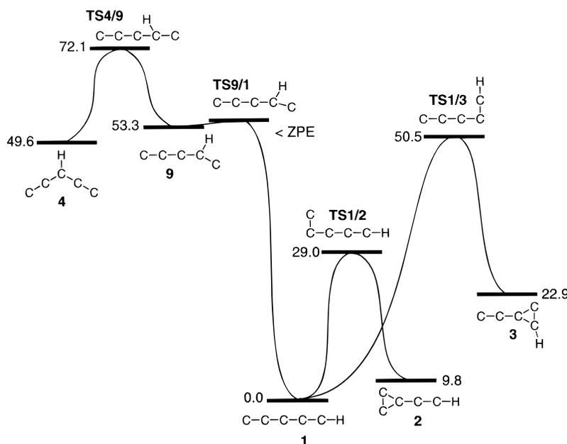
**Figure 2.** Reaction coordinate diagram for rearrangement processes occurring on the neutral radical  $C_5H$  potential surface. The geometries of all stationary points were calculated at the B3LYP/6-31G level of theory; those of the transition structures are available in Supporting Information. The relative energies were calculated using the same theory with the larger basis set, aug-cc-pVDZ, and are given in kcal mol<sup>-1</sup>, with zero-point energy contributions included.
