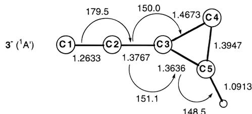
**Figure 4.** Optimized geometry for the singlet ground state of C<sub>2</sub>C<sub>3</sub>H<sup>-</sup> (3<sup>-</sup>). The geometry was calculated at the B3LYP/aug-cc-pVDZ level of theory. All bond lengths are given in angstroms and all angles in degrees.
