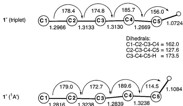
**Figure 1.** Optimized geometries for the singlet and triplet electronic states of  $C_4CH^-$  ( $1^-$ ). These geometries were calculated at the B3LYP/aug-cc-pVDZ level of theory. All bond lengths are given in angstroms and all angles in degrees.
