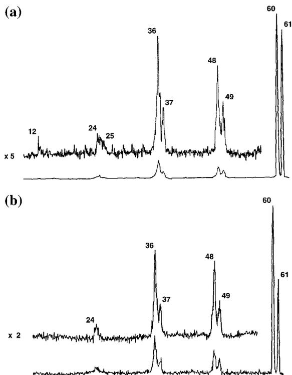
**Figure 7.**  $^{-}\text{NR}^+$  ( $\text{O}_2$ , 80% T;  $\text{O}_2$ , 80% T) spectra of  $m/z$  61 from (a)  $\text{TMSC}\equiv\text{CC}\equiv\text{CCH}_2\text{OCH}_3$ , giving  $\text{C}_4\text{CH}^-$ , and (b)  $\text{HC}\equiv\text{CCH}(\text{OCOCH}_2\text{-CH}_3)\text{C}\equiv\text{CH}$ , giving  $\text{C}_2\text{CHC}_2^-$ . These spectra both show fragments of the forms  $\text{C}_n\text{H}^+$  and  $\text{C}_n^{*+}$ .
