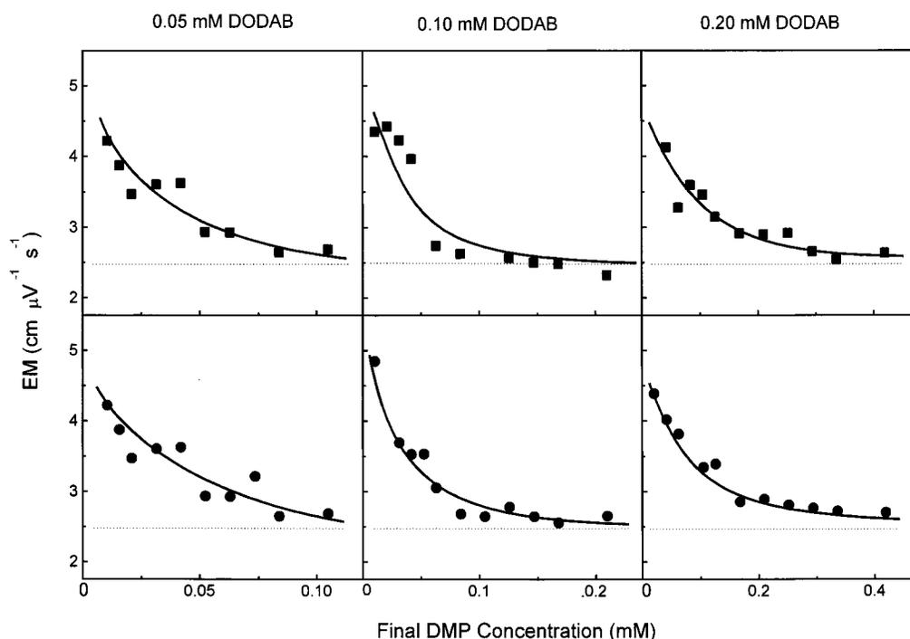
**Figure 5.** Electrophoretic mobilities (EM) of large DODAB vesicles as a function of final DMP concentrations in the mixtures for three different DODAB concentrations and two different vesicle preparation methods: Snippe's (■) or chloroform vaporization (●). Dashed lines indicate the leveling-off of EM (at ca. 2.5 of mobility) taking place at a final DMP concentration equal to approximately twice the DODAB concentration in each subfigure.
