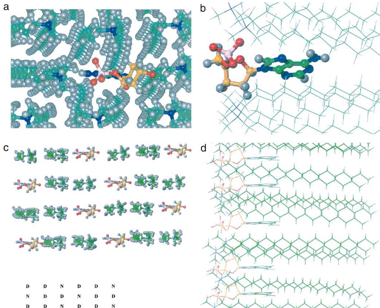
**Figure 6.** Three-dimensional representation of the energy-minimized nucleotide/DODAB complex: (a) top view below maximum adsorption; (b) cross-section below maximum adsorption; (c) top view at maximum nucleotide adsorption (notice the molar ratio DODAB:DMP equal to 2:1); (d) cross-section at maximum nucleotide adsorption. For the sake of clarity, carbon atoms of riboses are shown in orange. In (c), D represents DODAB and N, the nucleotide.
