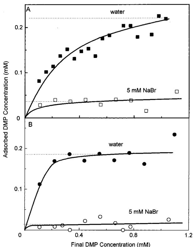
**Figure 2.** The effect of 5 mM NaBr on DMP adsorption onto large DODAB vesicles either obtained by Snippe's method in water (■) or 5 mM NaBr (□) or obtained by the chloroform vaporization in water (●) or 5 mM NaBr (○). The final DODAB concentration in each mixture is 0.5 mM.
