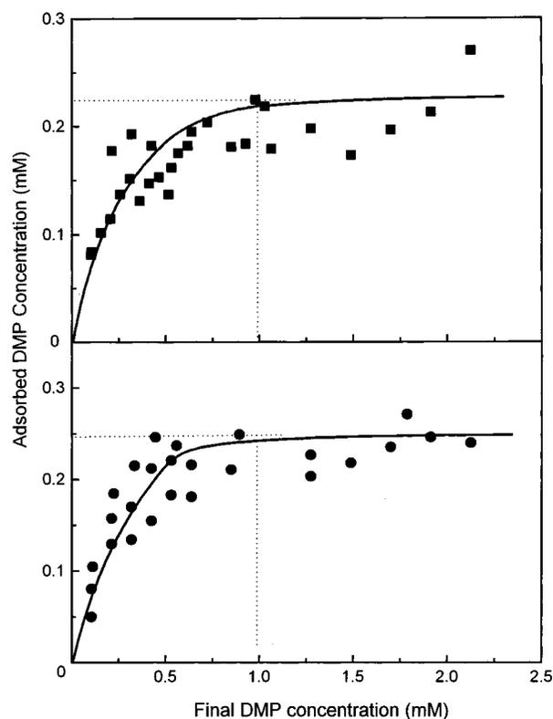
**Figure 1.** Adsorption isotherm for the adsorption of DMP from water solution onto large DODAB vesicles. Vesicles were obtained by Snippe's (■) or by the chloroform vaporization method (●). One should notice that maximal adsorption is achieved approximately at the point indicated by dashed lines. The DODAB:DMP molar proportion at this point is ca. 2:1, as also depicted from linearization of the isotherms in Table 1.
