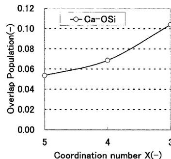
**Figure 6.** Bond overlap population between Ca and O in the  $\text{Ca}(\text{OH})_x^{(x-2)}-\text{SiO}_4\text{H}_3^{3-}$  cluster.
