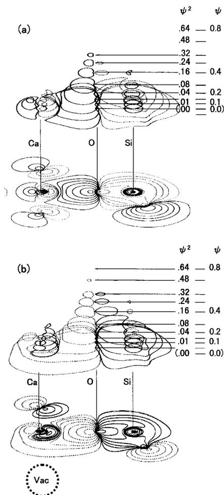
**Figure 4.** Contour maps of the bonding molecular orbitals for Ca, O, and Si in the  $\text{CaO}_4^{(2x-2)}-\text{SiO}_4^{4-}$  cluster and the amplitude of their wave function  $\psi$ . Different lines represent different phases: (a)  $x = 5$  (surface). (b)  $x = 4$  (surface with an oxygen vacancy).
