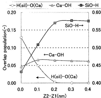
**Figure 5.** Bond overlap population between  $\text{H}(X_1, Y_1, Z_1)$  and  $\text{O}(X_2, Y_2, Z_2)$  in the  $\text{Ca}(\text{OH})_6^{4-}-\text{SiO}_4\text{H}_2^{2-}$  cluster at  $Z_2-Z_1 = 0$ ,  $\text{H}-\text{O}$  length 0.1 nm.
