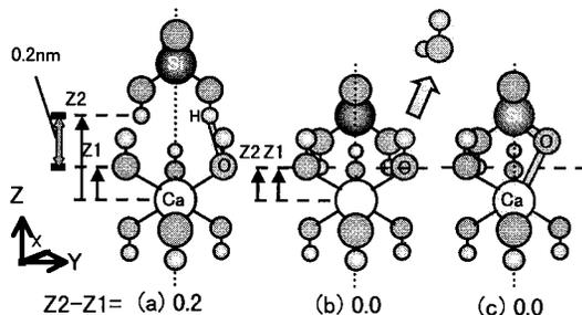
**Figure 2.**  $\text{Ca(OH)}_6^{4-}\text{--SiO}_4\text{H}_2^{2-}$  cluster calculated for the  $\text{Ca(OH)}_2\text{--SiO}_2$  interface: (a) the difference in the Z coordinates,  $Z_2\text{--}Z_1$ , is 0.2 nm, (b)  $Z_2\text{--}Z_1 = 0.0$  nm. (c)  $\text{Ca(OH)}_x^{(4-2x)-}\text{--SiO}_4\text{H}_1^{3-}$  cluster after the dehydration at  $Z_2\text{--}Z_1 = 0.0$ . A Ca–O–Si bond is formed.
