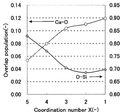
**Figure 3.** Bond overlap population between Ca and O, and O and Si in the  $\text{CaO}_x^{(2x-2)-}\text{--SiO}_4^{4-}$  cluster.
