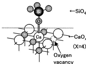
**Figure 1.**  $\text{CaO}_x^{(2x-2)-}\text{--SiO}_4^{4-}$  cluster calculated for the CaO–SiO<sub>2</sub> interface.
