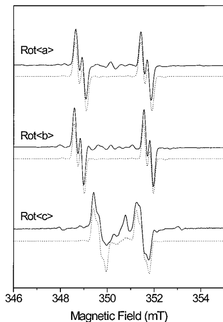
Figure 8. Experimental (solid lines) and simulated (dotted lines) EPR spectra from malonic acid at room temperature. The microwave power is 0.5 mW, and the modulation frequency is 6 kHz at a width 0.11 mT. The orientations of the magnetic field are as follows: (a) 150.8° from the reference zero point in the rot(a) plane, corresponding to polar angles \theta = 51.5^\circ and \varphi = 33.0^\circ ; (b) same as Figure 3; and (c) 125.6° from the reference zero point in the rot(c) plane, corresponding to polar angles \theta = 90.0^\circ and \varphi = -54.4^\circ .
