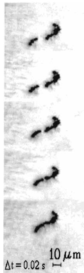
Figure 8. Imaging system results illustrating collisions between silicon agglomerates. The picture is represented by a series of frames separated by a time interval, \Delta t = 0.02 \text{ s} . Time increases from top to bottom. Reactor temperature, T = 873 \text{ K} . Cold-zone coagulation time, t = 10 \text{ s} .
