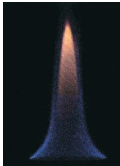
Figure A-2. Photograph ( f/2.4 , 1/60 s) of DME Meeker burner diffusion flame. DME volume flow = 330 \text{ cm}^3 \text{ min}^{-1} .
