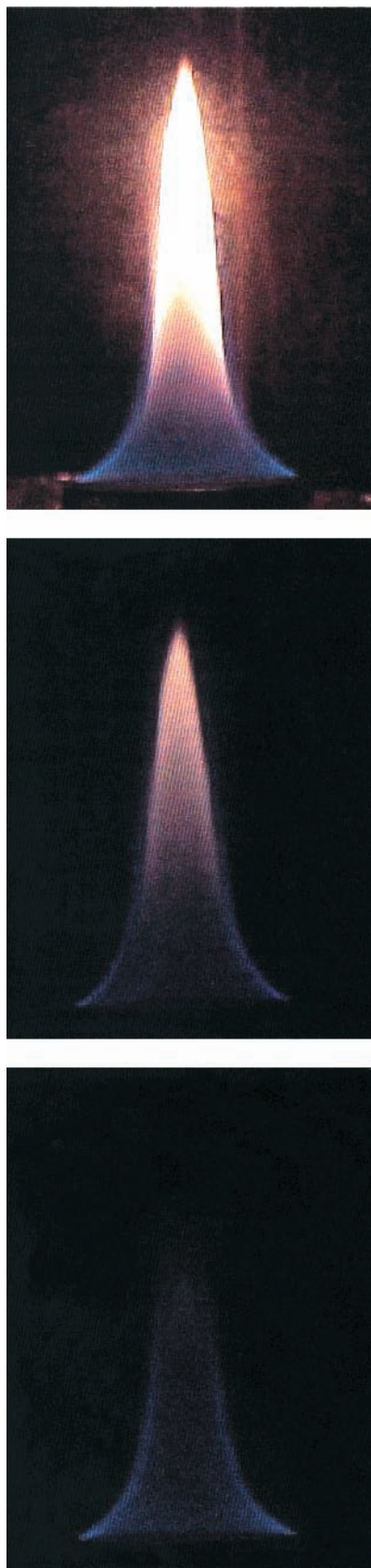
Figure A-3. Photographs ( f/2.4 , 1/60 s) of Meeker burner diffusion flames: top = ethane ( 220 \text{ cm}^3 \text{ min}^{-1} ); middle = methane ( 440 \text{ cm}^3 \text{ min}^{-1} ); bottom = DME ( 215 \text{ cm}^3 \text{ min}^{-1} ).
