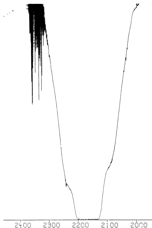
Figure 2. Infrared spectrum of \text{DSM-}d_0 in the \nu\text{SiH} region, showing combination and difference bands involving torsional frequencies. Partial pressure of sample, 70 Torr in a 12 cm cell.
