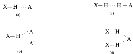
(a) single hydrogen bridge (bond) (c) dihydrogen bond [15] (b) bifurcated hydrogen bridge (d) twofold hydrogen bridge
