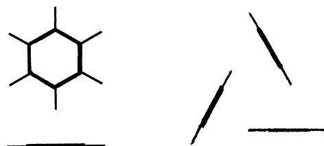
Figure 1. Equilibrium geometries of the T-shaped ( C_{2v} ) benzene dimer and cyclic ( C_{3h} ) trimer of naphthalene, as deduced from the microwave spectroscopy 1 and rotational coherence spectroscopy, 2 respectively.
