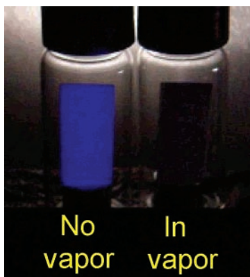
Figure 4. On-off fluorescence switching of TPBD thin layer developed on the TLC plate without vapor (left) and in vapor (dichloromethane) (right) under UV light (365 nm) illumination at room temperature.
