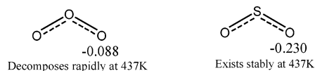
Figure 2. The ESP charges of oxygen atoms in O_3 and SO_2 , and their thermal stabilities.
