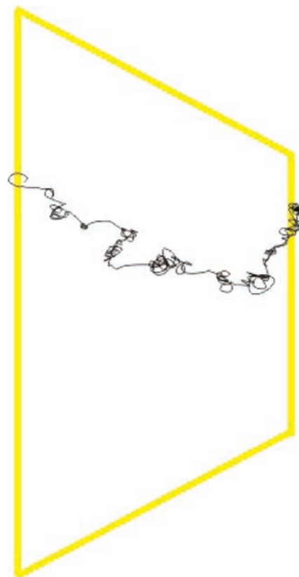
Figure 5. The trajectory of a liquidlike atom diffusing from the internal to the external surface across the percolating network at GBs. Data are extracted from an atomic configuration at 1158 K.
