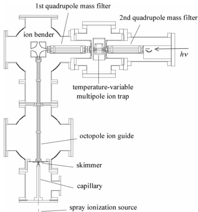
**Figure 1.** Schematic drawings of the experimental apparatus.
