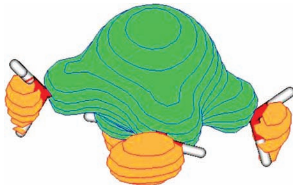
Figure 2. Contour plot of the 13th orbital. This orbital was built by a mixture of the 6s^2 lone pair of electrons of the lead with the nonbonding (O, 2p) lone pairs of the water molecules.
