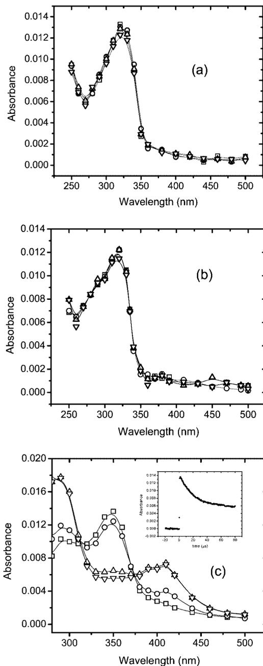
**Figure 2.** Transient absorption spectra obtained from electron pulse radiolysis of  $N_2O$ -saturated solutions of penicillin G (a), penicillin V (b), and amoxicillin (c): 1 ( $\square$ ), 5 ( $\circ$ ), 50 ( $\Delta$ ), and 100  $\mu$ s ( $\nabla$ ). The insert on c shows the decay trace of the intermediate of amoxicillin observed at 350 nm.
