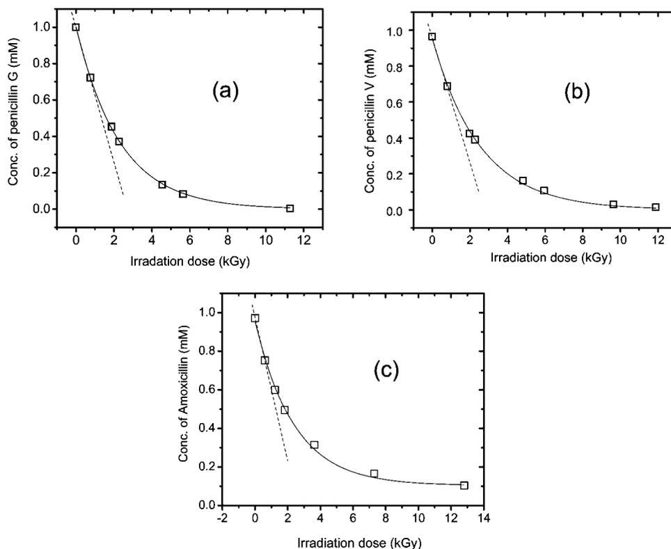
**Figure 6.** Measured loss of penicillin G (a), penicillin V (b), and amoxicillin (c) in aerated aqueous solutions using  $^{137}\text{Cs}$   $\gamma$  irradiation. Curves correspond to fitted exponential loss, while dashed straight lines are the estimated initial slope values of  $k = -3.69 \times 10^{-4}$ ,  $-3.47 \times 10^{-4}$ , and  $-3.71 \times 10^{-4} \text{ M kGy}^{-1}$  for penicillin G, penicillin V, and amoxicillin, respectively.
