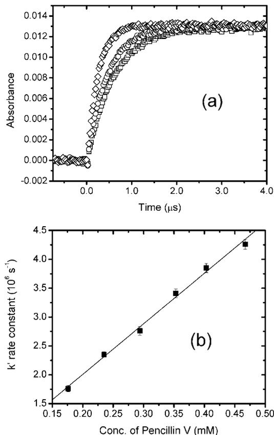
**Figure 3.** (a) Typical growth kinetics of transient absorption at 320 nm in a pulse-irradiated solution at pH 7.0 and room temperature for 0.467 ( $\diamond$ ), 0.235 ( $\circ$ ), and 0.176 ( $\square$ ) mM penicillin V. (b) Second-order rate constant determination for the reaction of hydroxyl radicals with penicillin V at 320 nm ( $\blacksquare$ ). Solid line corresponds to the value of the overall rate constant  $k = (8.76 \pm 0.28) \times 10^9 M^{-1} s^{-1}$ .
