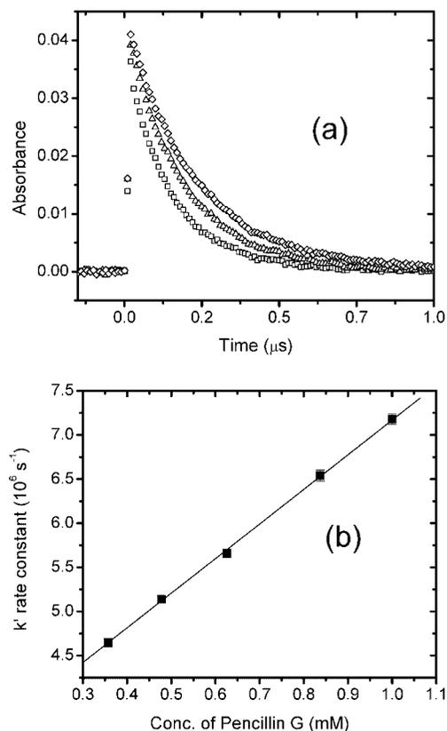
**Figure 5.** (a) Typical decay kinetics for hydrated electron reduction (measured at 700 nm) for 1.00 ( $\square$ ), 0.626 ( $\Delta$ ), and 0.357 ( $\diamond$ ) mM penicillin G at pH = 7.0 and room temperature. (b) Second-order rate constant determination for reaction of the hydrated electron with penicillin G. The straight line is the weighted linear plot with a slope of  $3.92 \pm 0.10$ .
