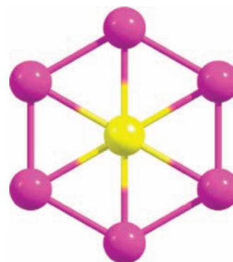
Figure 1. Molecular geometry of planar (B_6C)^{-2} dianion. The pink spheres represent boron atoms, whereas the central yellow one represents the carbon atom.
